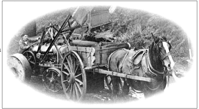
Image Above: The first tractor powered front-end loader made in Australia. Designed and built by Malcolm Moore circa 1925. Source: Malcolm Moore Golden Jubilee
