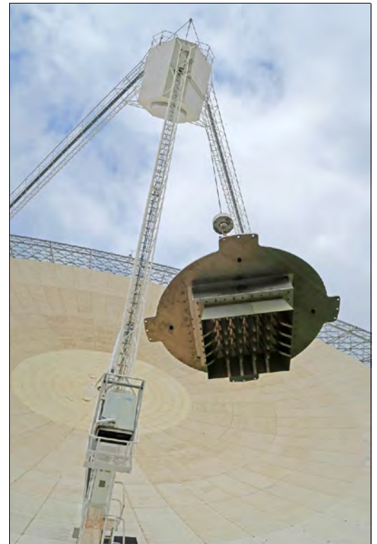
Lifting the prototype cryogenically cooled Phased Array Feed (PAF) into the focus Cabin for testing in 2016. Photo: John Sarkissian.
